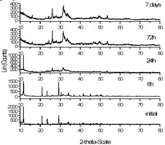
Fig. 1: Diffractograms of dried sample of brushite, which stayed for 6, 24, 72 hours and 7 days in SBF.
